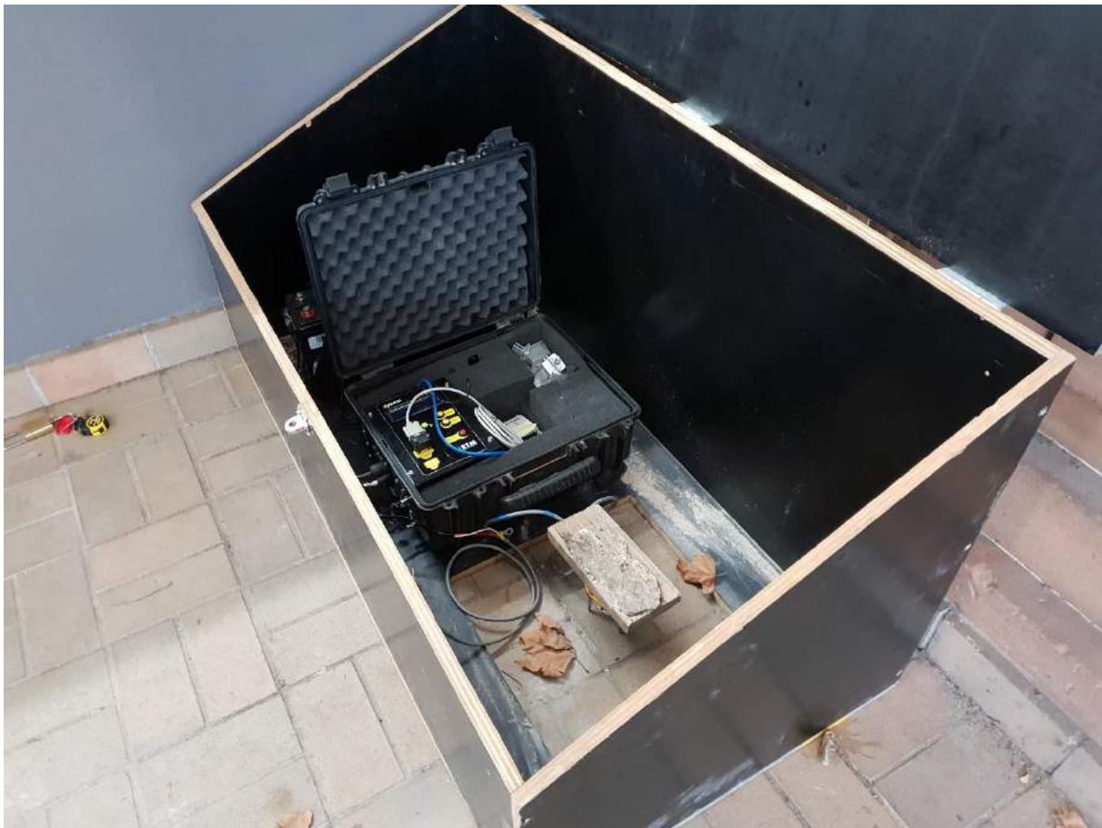
Figure 2-8: Real time vibration logger Central Electric Building
