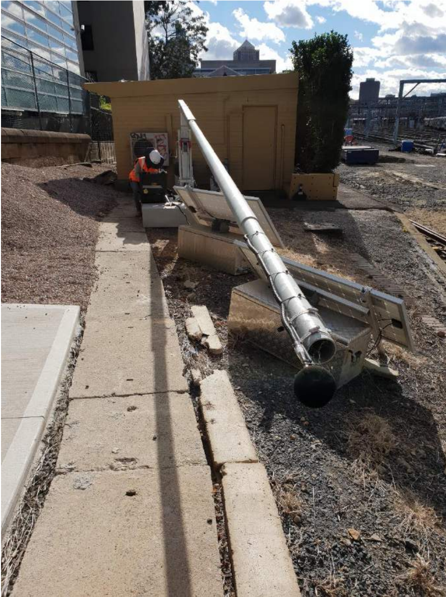
Figure 2-5: Real time noise logger setup at 54 Regent St (in the process of being serviced)
