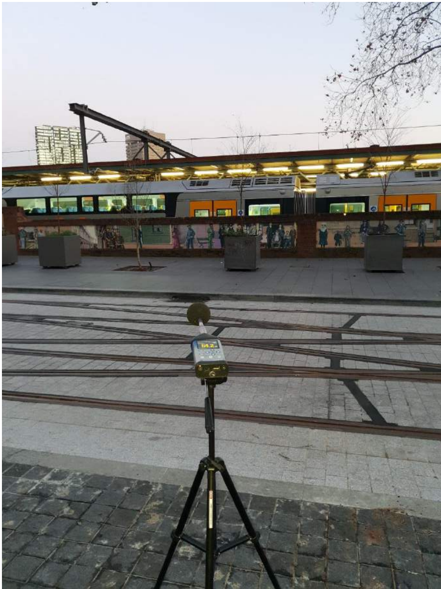
Figure 2-3: Attended noise logger setup on Chalmers St
