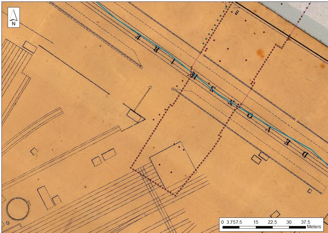
Figure 61: Central Station Main Works station box overlain on the 1884 Waterboard Survey plan Sheet S2
