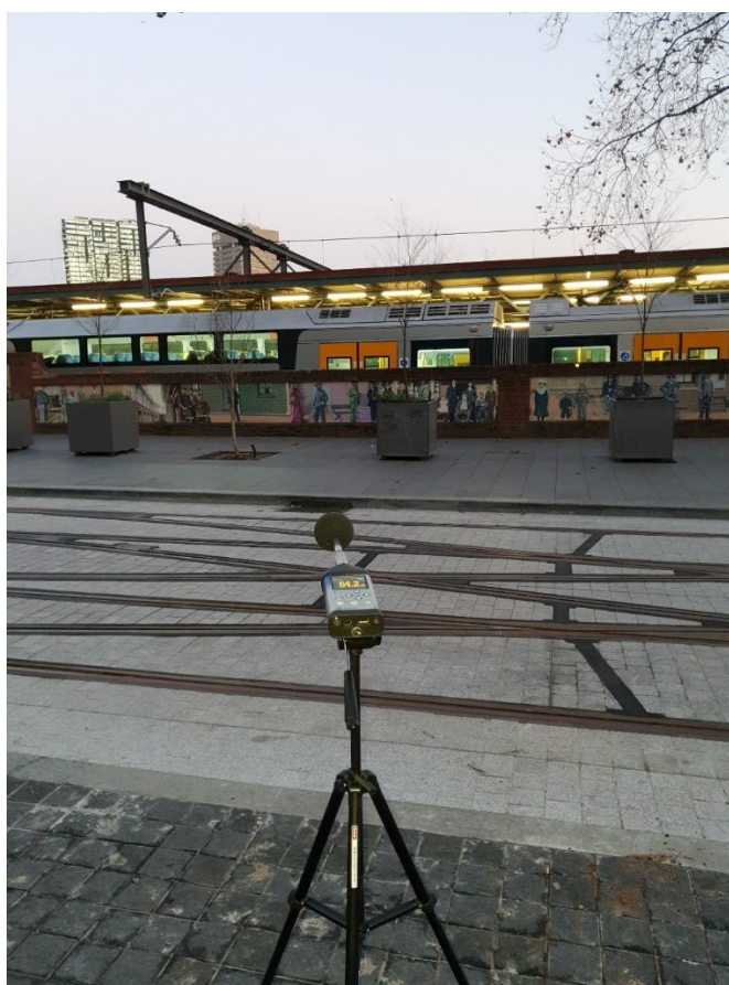
Figure 2-3: Attended noise logger setup on Chalmers St
