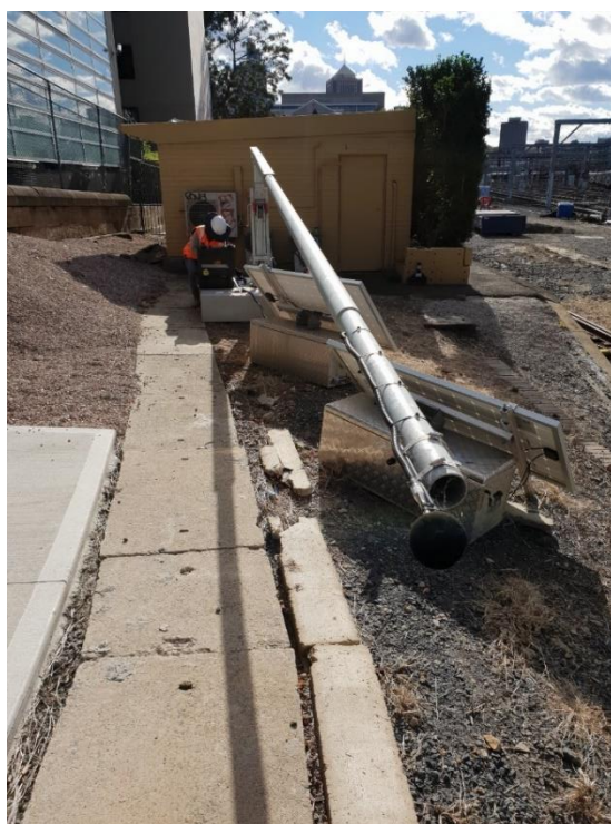
Figure 2-5: Real time noise logger setup at 54 Regent St (in the process of being serviced), installed 12/12/2018
