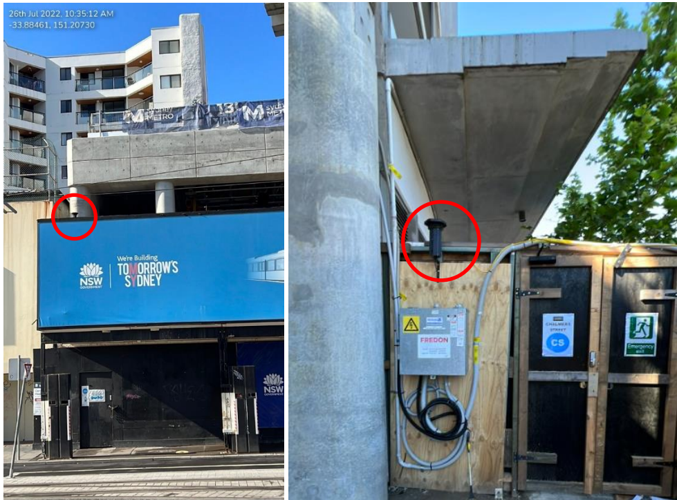
Figure 2-4: Real time noise logger Chalmers St used at different locations during the reporting period.
