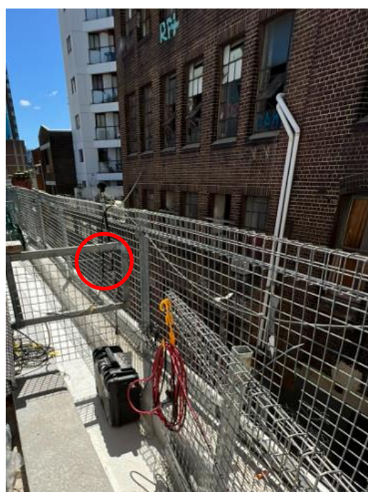
Figure 2-3: Real time noise logger setup at 20-28 Chalmers St (Randle Lane side)
