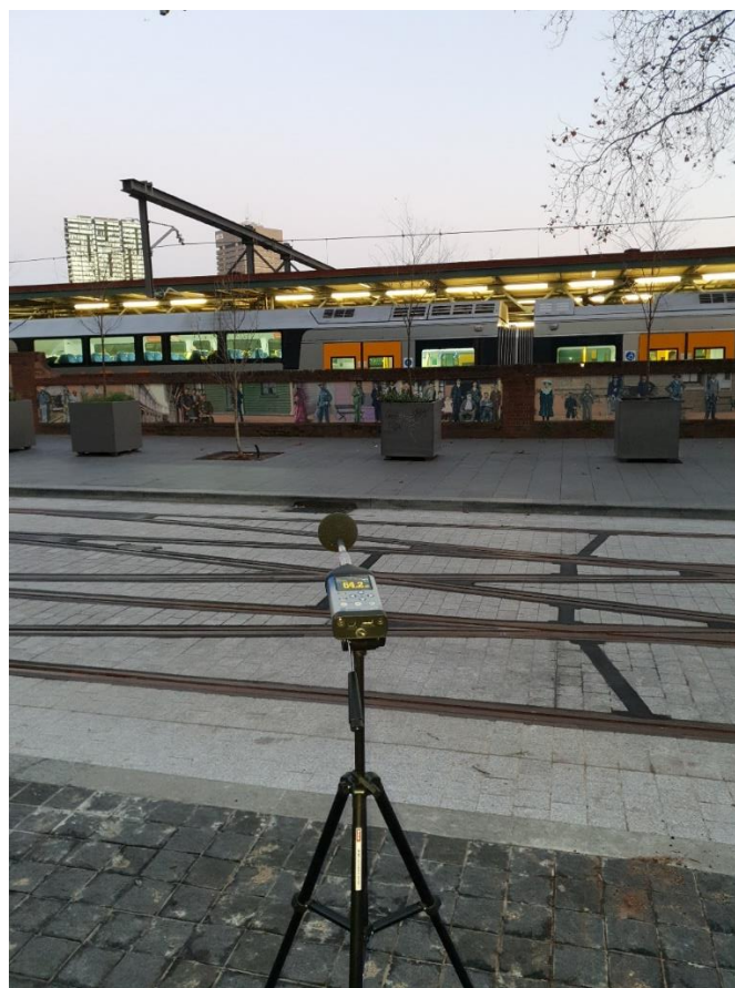
Figure 2-2: Attended noise logger setup on Chalmers St
